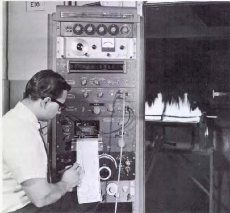
Figure 3. Test assembly for fire-resistant cables.
