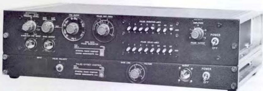
Figure 1. Panel view of the Type 1394-Z High-Rate Pulse Generator, consisting of (top) the Type 1394-A High-Rate Pulse Generator and (bottom) Type 1394-P1 Pulse-Offset Control.
