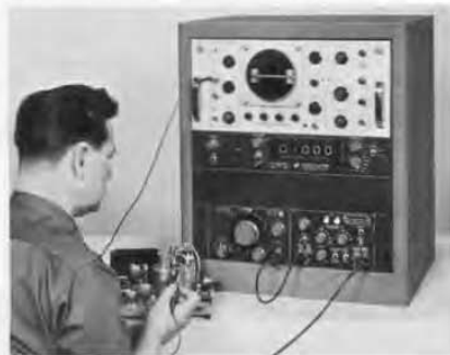
Figure 15. Rack-mounted Type 1310-A Oscillator and Type 1396-A Tone-Burst Generator used to test amplifier overload characteristics. A behind-the-panel connection to the synchronization jack allows precise readout of frequency on the Type 1150-B Digital Frequency Meter.
