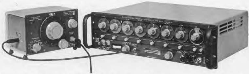
Figure 6. The Type 1310-A Oscillator with a Type 1161-A7C Synthesizer used as an adjustable high-accuracy, high-voltage, low-distortion source for a precision fm-deviation measurement. The output frequency, 31.063 kc/s, when used to modulate an fm generator produces a null in the carrier for a \pm 75.00 -kc frequency deviation.
