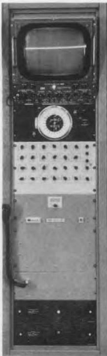
(Right) Group of fairgoers listening attentively to the satellite-tracking demonstration. (Left) Close-up view of the center rack. The Synchronometer with its 24-hour clock face is near the top; the standard-frequency oscillator and frequency divider are at the base.
