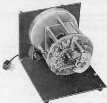
Figure 3. Rear view of the Unit Oscillator, with cover removed, showing tuned circuit inductors and sickle-shaped cores.
