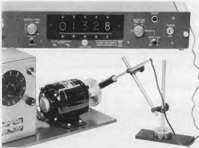
Figure 2. The Photoelectric Pickoff shown with the Type 1150-A Digital Frequency Meter (top), as arranged to measure the speed of an electric motor.
