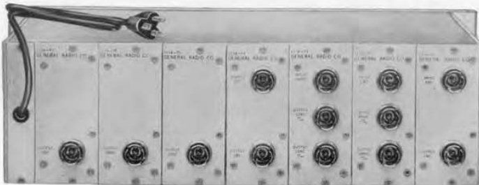
Figure 8. Rear view of the divider with plug-in units installed.
