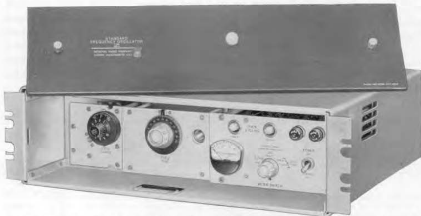
Figure 5. View of Type 1113-A Standard-Frequency Oscillator control panel. The front panel is held in place with two catches, and is easily removed for adjustment of controls or observation of oven performance. The meter can be switched to perform any one of several functions, as a diagnostic device. The coarse and fine frequency controls cover a total range of adjustment of 5 \times 10^{-7} yet permit setting to 10^{-10} . The fine control is direct-reading, with divisions spaced at intervals of 5 \times 10^{-10} .
