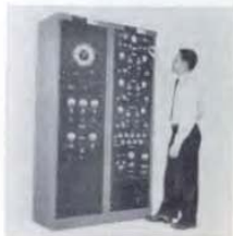
View of the new Type 1120-AH 1000-Mc Frequency Standard (left-hand rack) with the Type 1105-B Frequency Measuring Equipment (right).
