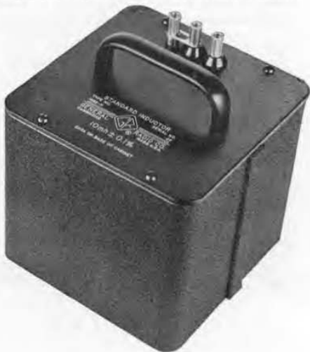
Figure 1. A stable low-frequency inductance standard, the General Radio Type 1482 Standard Inductor.
