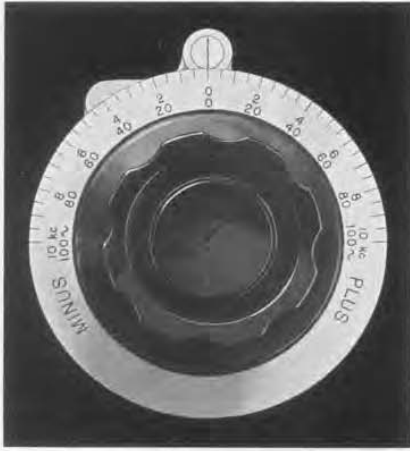
FIGURE 5. The CYCLES INCREMENT dial, shown here, carries two scales, one for each output frequency range of the oscillator. The range is \pm 10 kc for the high-frequency range and \pm 100 cycles for the low range.
