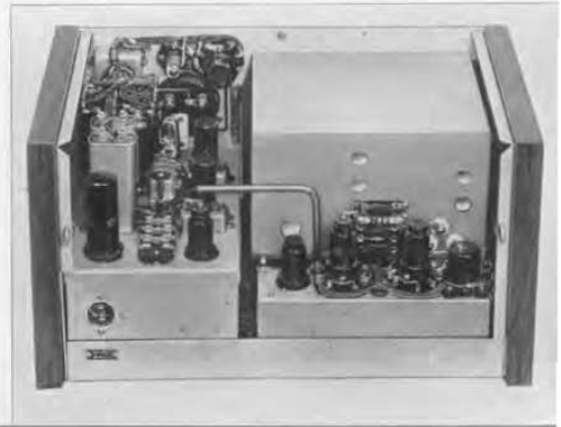
FIGURE 4. Rear view of the oscillator, showing details of construction. The wooden end pieces can be removed when the instrument is to be mounted in a relay rack.
