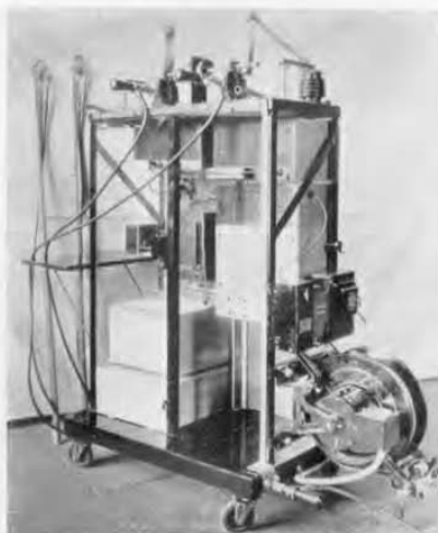
FIGURE 2. Rear view of the equipment, showing the type of construction used. The beat-frequency oscillator and power amplifier were designed and manufactured by the General Radio Company. The recording equipment, motor drive, and the protective and coupling devices were built by the Pennsylvania Water and Power Company
