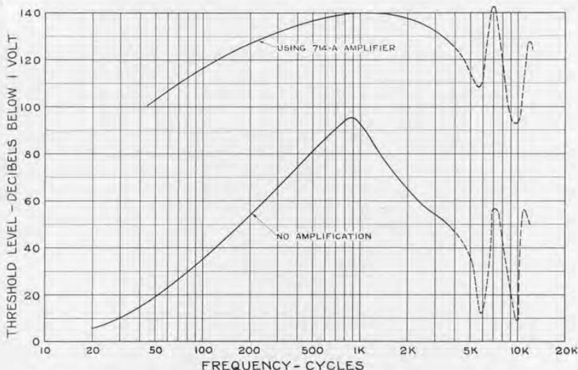
FIGURE 6. Plots showing how TYPE 714-A Amplifier improves the frequency characteristic in bridge measurements
