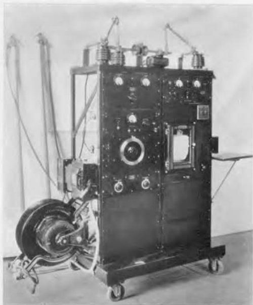
FIGURE 1. Panel view of the fault-locating equipment, showing the beat-frequency oscillator, power amplifier, and recorder
